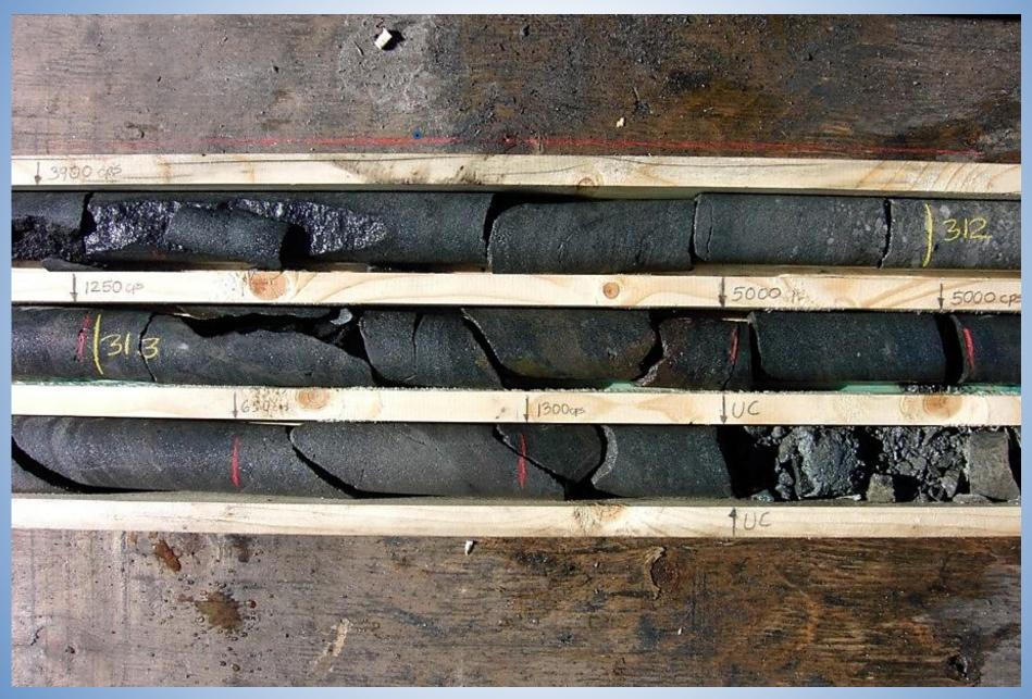
Mineralized Intersection in Black Lake hole BL-18 - 0.69% U<sub>3</sub>O<sub>8</sub> over 4.4m
